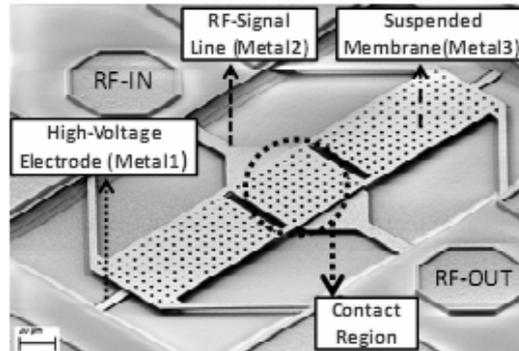
**Fig. 1.** BiCMOS embedded RF-MEMS switch [6].
