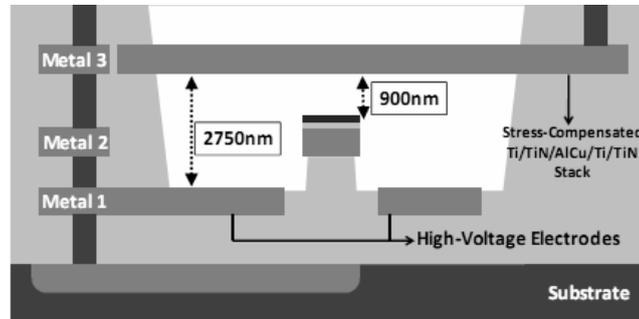
Fig. 3. Detailed cross-section of the RF-MEMS varactor.
