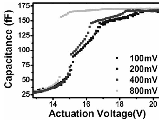
**Fig. 7.** De-embedded contact capacitance versus actuation voltage curves for different amplitudes of AC signal used for capacitance measurements. Every point shows a measurement point with an increment of 100mV.
