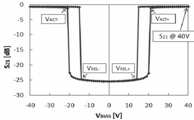
Fig. 2.  $S_{21}$  parameter vs. bias voltage for a typical device.
