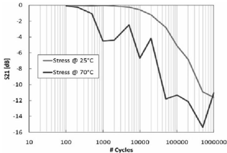
**Fig. 5.** Average  $S_{21}$  parameter vs. number of cycles of the same device cycled at different temperatures. The higher the temperature, the faster a switch is damaged. The  $S_{11}$  parameter, shows the same behavior.
