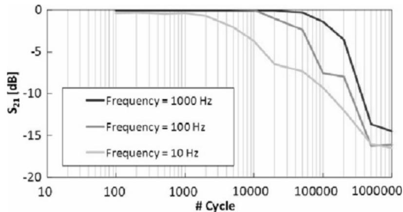
**Fig. 6.** Cycling tests performed at different frequencies. The charge trapping effect appears stronger at lower frequency than the one at higher frequency.
