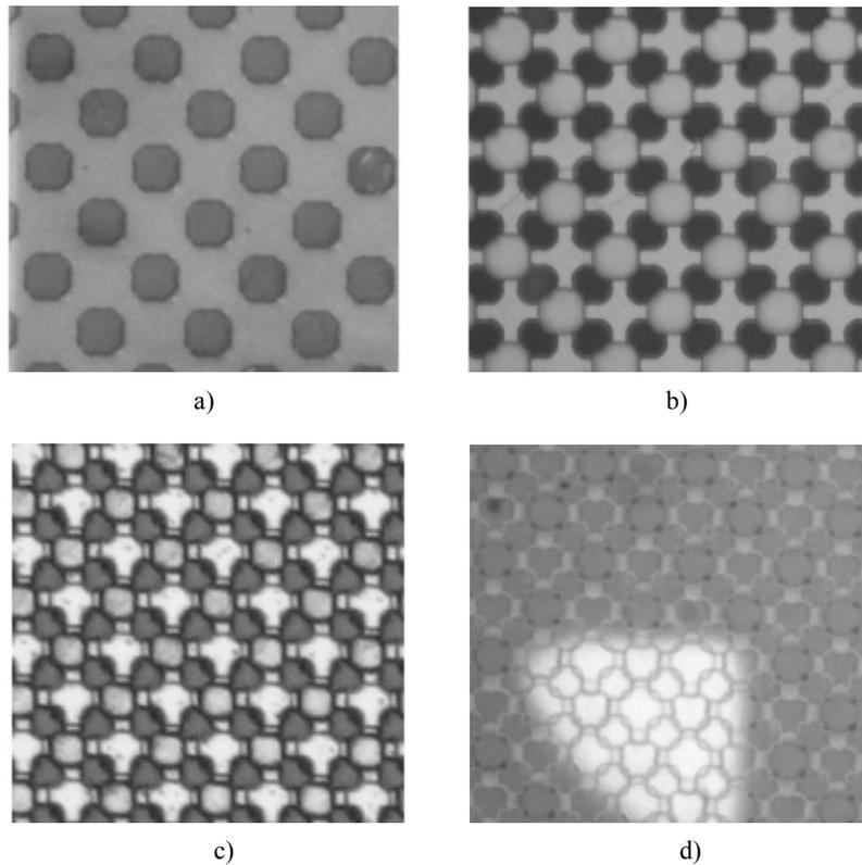
**Fig. 3.** Pictures of holes distribution at different process stages: a) First PECVD nitride layer. b) Sacrificial aluminum layer. The dark areas are the holes in this layer. c) Second PECVD nitride layer. The holes in this layer are centered on the cyan crosses, while the light green squares correspond to the holes in the first nitride layer. d) Final released structure. The light area is an underlying aluminum pattern.
