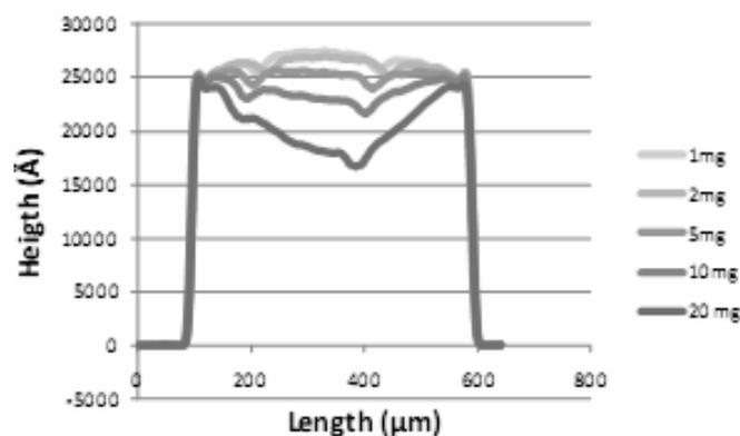
Fig. 5. Load test of a  $500\mu\text{m}$  wide released nitride shell.
