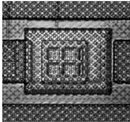
Fig. 4. Cantilever switch included in the nitride cage.
