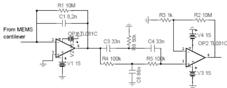
Fig. 8. Charge amplifier schematic.
