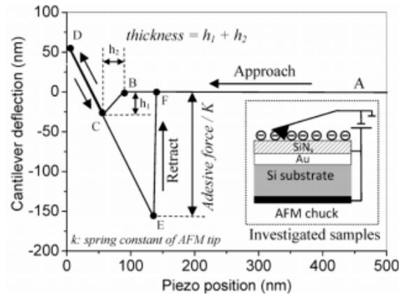
Fig. 1. Force-distance curve for the investigated samples.
