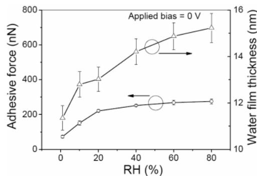
**Fig. 2.** The influence of the relative humidity on adhesive force and adsorbed water film thickness.
