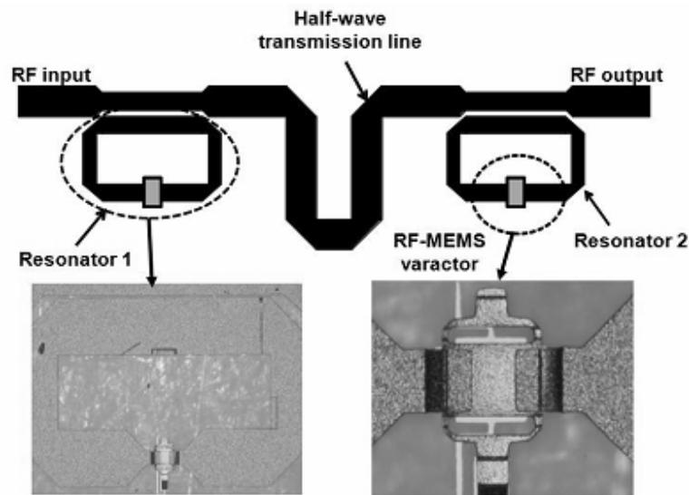
**Fig. 1.** Design of the 2 pole tunable X-band rejecter filter based on RF-MEMS varactor.
