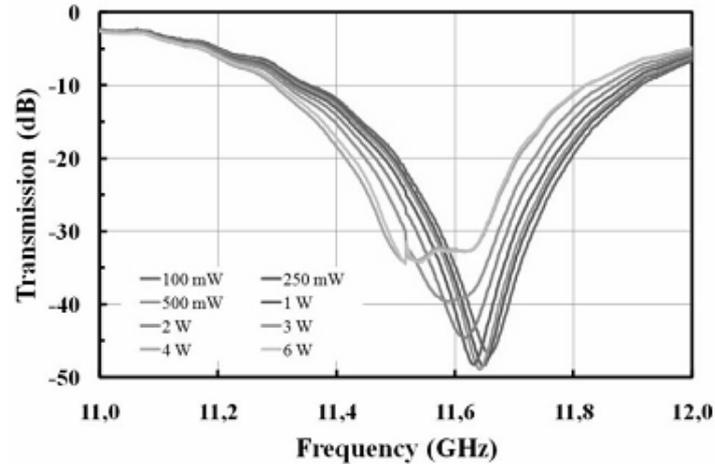
Fig. 7. Influence of RF power on rejection when RF MEMS are in the down state.
