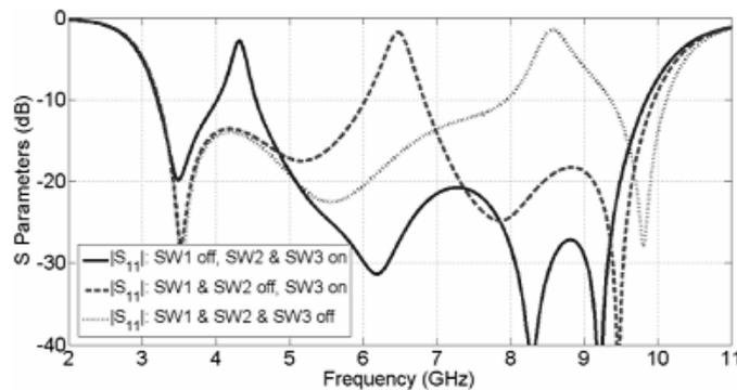
Fig. 7. Comparison among the UWB filter  $|S_{11}|$  responses of the three different stub configurations (HFSS®).
