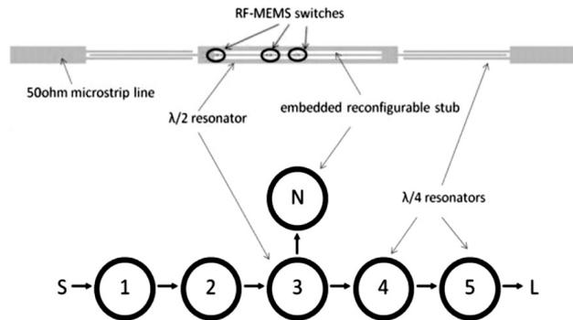
**Fig. 1.** Layout and scheme of the UWB bandpass 5<sup>th</sup> order filter.
