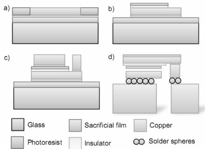
**Fig. 3.** Fabrication process flow for the MEMS varactor.
