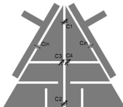
**Fig. 1.** Layout of the selectable multiband triangular patch filter.
