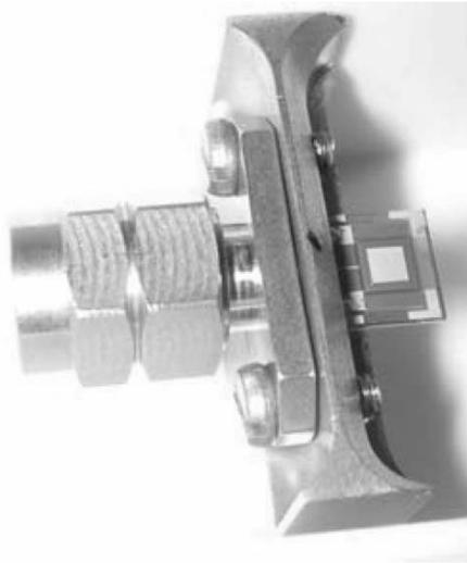
**Fig. 5.** Prototype antenna mounted on V-connector.
