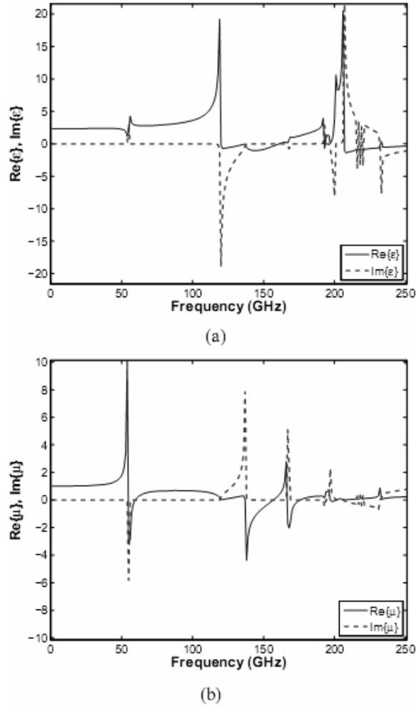
**Fig. 6.** Left-handed performance at the actuation voltage of 0 V.
