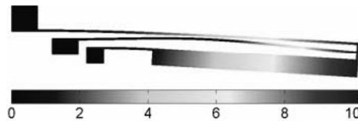
**Fig. 3.** Total displacement distribution on the actuator (in  $\mu\text{m}$ ) at the actuation voltage of 15 V.
