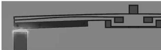
**Fig. 14.** Electric field snapshot of the double parallel actuated device at 58 GHz.
