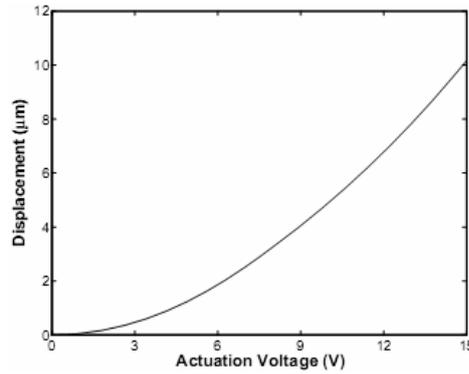
**Fig. 2.** Maximum tip displacement for different values of the actuation voltage.
