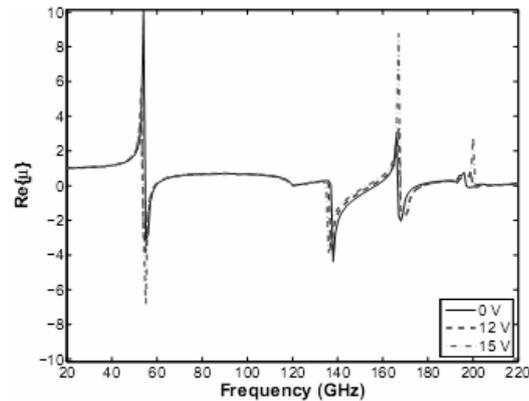
**Fig. 9.** Tunable left-handed performance at several actuation voltages in terms of effective magnetic permeability.
