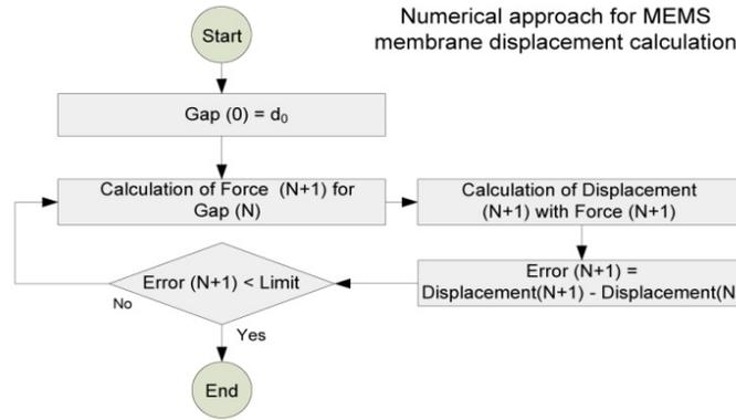
Fig. 2. Numerical approach of the MEMS membrane displacement calculation.
