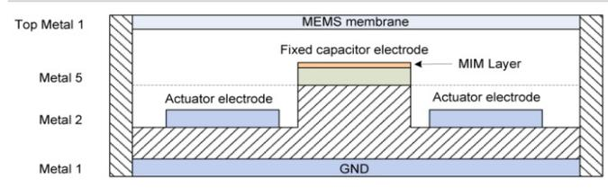
**Fig. 4.** (Color on line). MEMS varactor configuration within the IHP SG13 BEOL metal stack.
