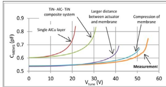
**Fig. 5.** (Color on line). Measured and simulated CV curves successively including the composite MEMS membrane layer system and the inherent deflection of the membrane.
