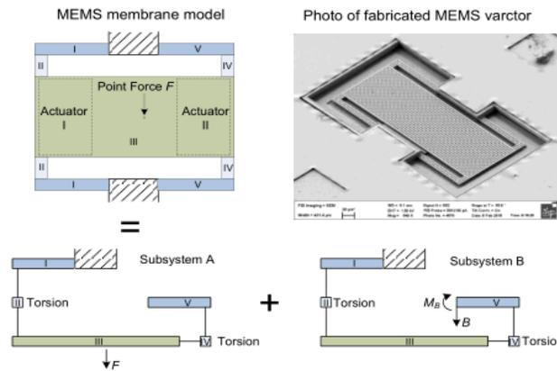
**Fig. 1.** (Color on line). Model of MEMS membrane and photo of the fabricated MEMS varactor.
