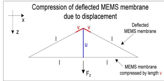
**Fig. 3.** Compression of deflected MEMS membrane when displaced by a distance  $u$  and a force  $F$ .
