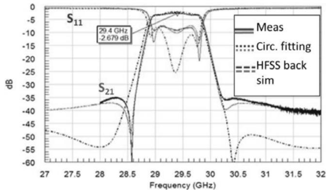
Fig. 8. RF measurements compared with circuital (AWR) and HFSS back simulation, accounting for the actual cavity dimensions.
