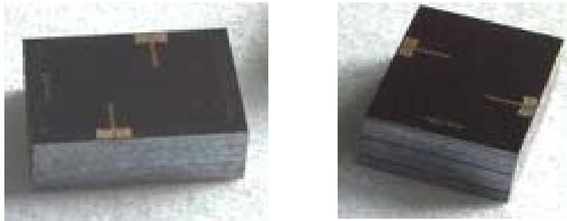
**Fig. 6.** Pictures of fabricated 4th pole filters.
