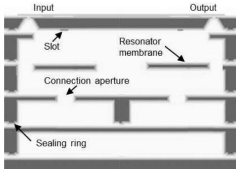
Fig. 2. Schematic cross section of a filter showing the 6 layers.
