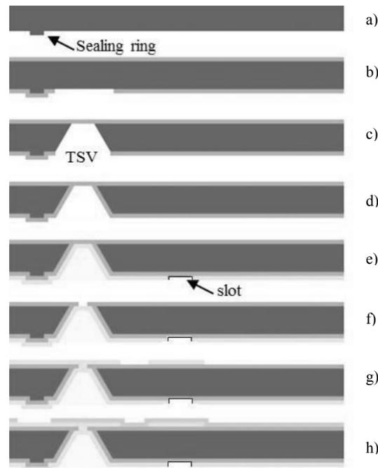
**Fig. 3.** Processing sequence for the top layer of the Ka band filter.
