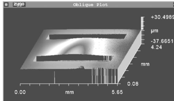
Fig. 7. Optical profiler measurement of a resonator membrane showing a slight deflection of a few microns.
