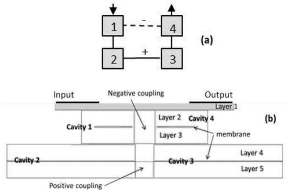
Fig. 1. 4<sup>th</sup> order Ka band filter topology (a) and schematic cross section (b).
