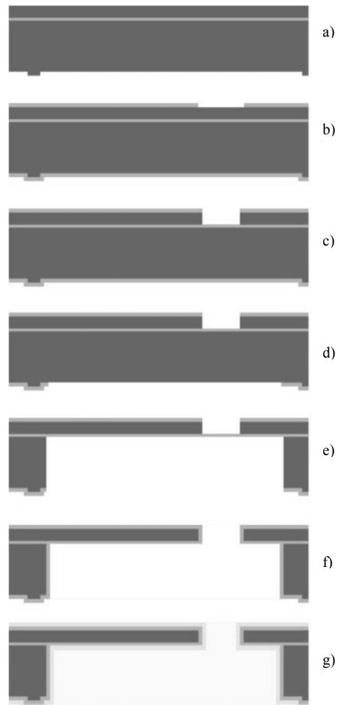
**Fig. 4.** Processing sequence for the middle layers of the Ka band filter.
